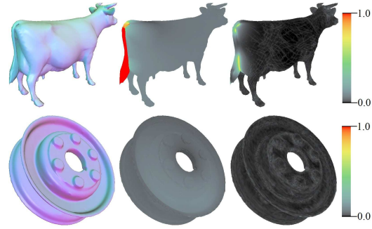
Figure 7: Examples of how the Poisson solver can fail due to thin regions in the surface (middle) and how regularization can help alleviate the problem (right).
